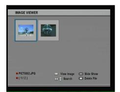
The figure on the left is a running screen of a TAP, *Image Viewer*, which displays image files of BMP, GIF and JPG format. This TAP is available from the web site, http://www.i-topfield.com.
